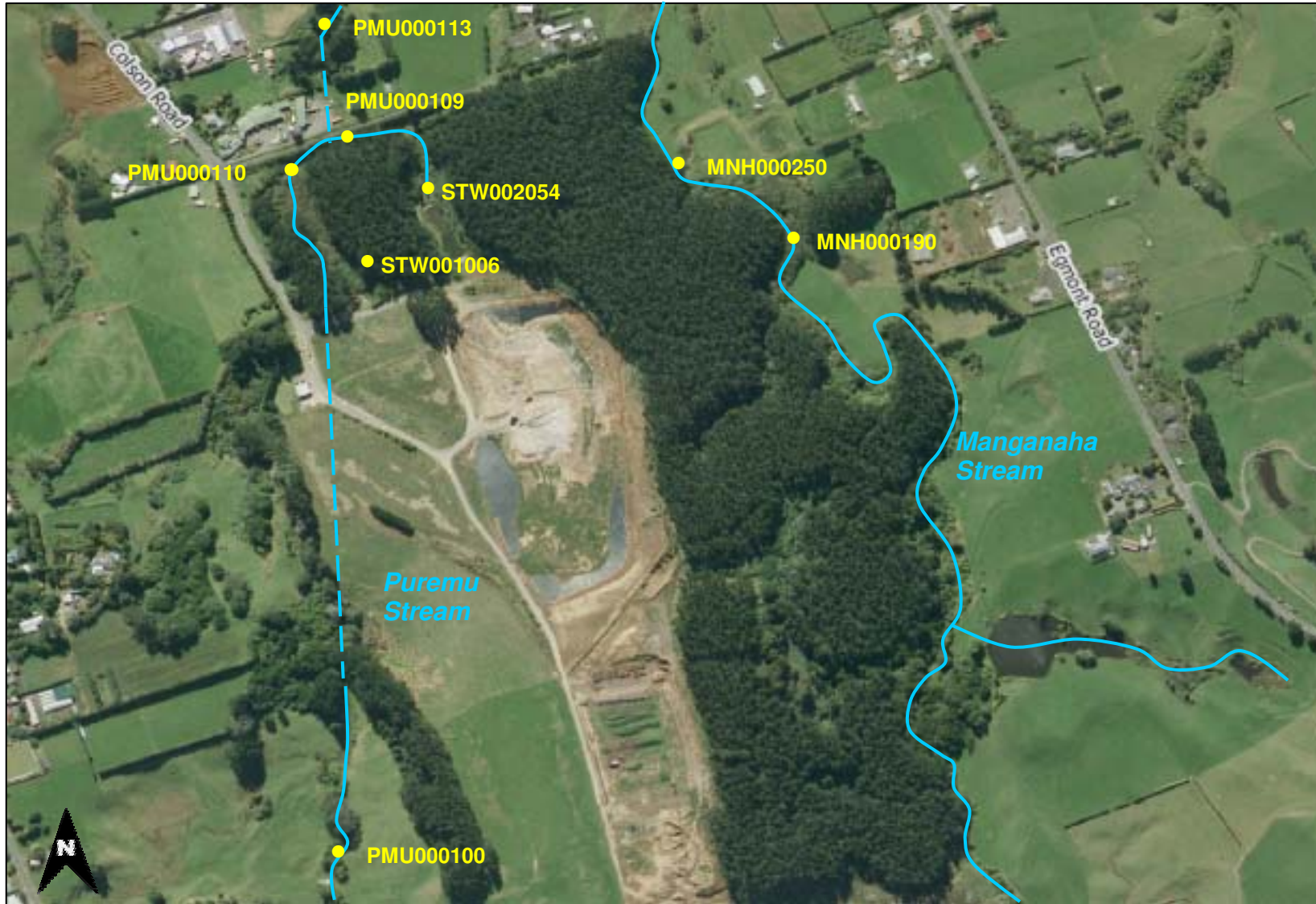
Figure 2 Aerial photo showing the stormwater and receiving water sampling sites at Colson Rd landfill
