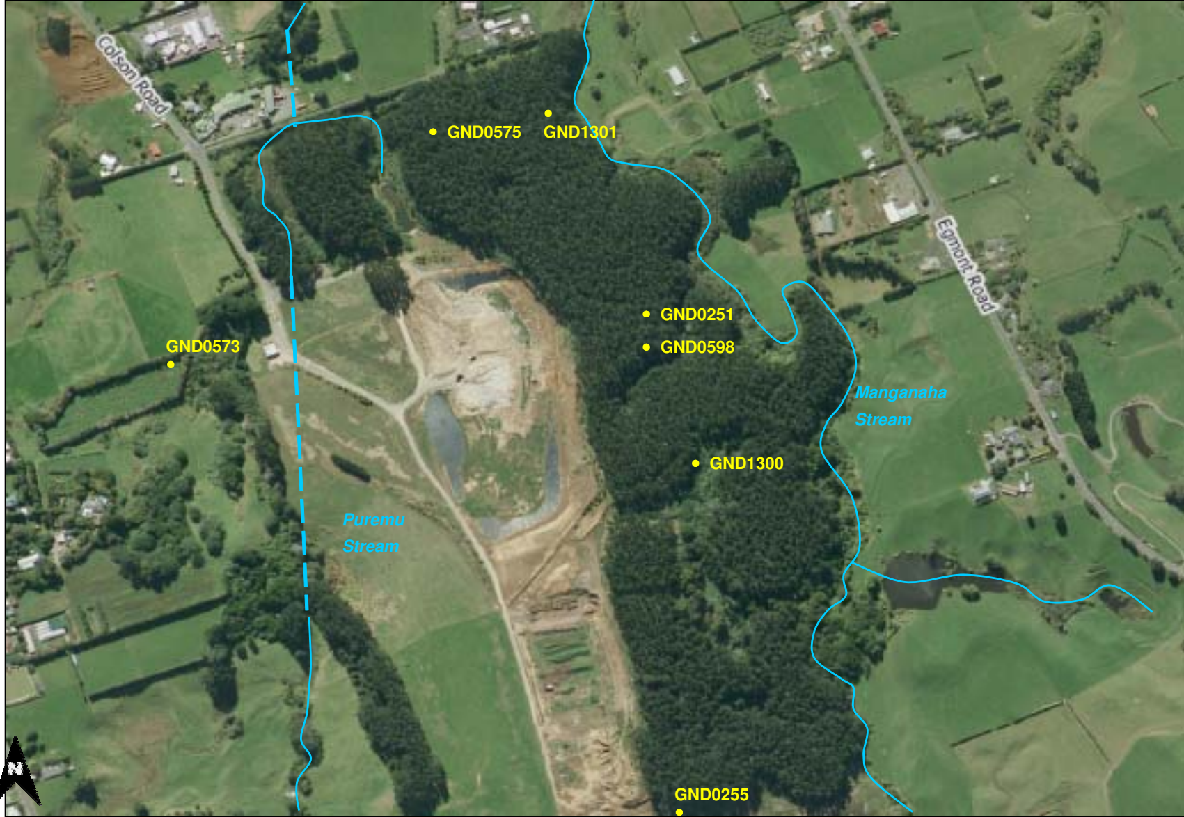
Figure 3 Aerial view of Colson Rd landfill showing the positions of groundwater monitoring bores
