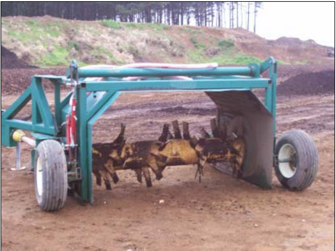
Photograph 3 Specialist compost turning machine at Colson Rd landfill, 28 October 2008
