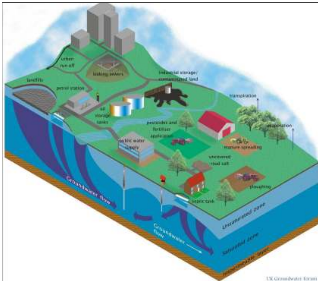
Figure 1 Sources of groundwater contamination 2
