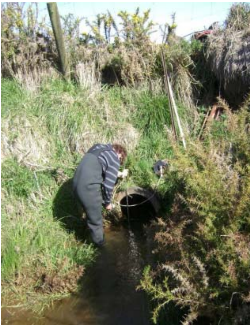
Photo 4 Installation of a staff gauge at a new control point
