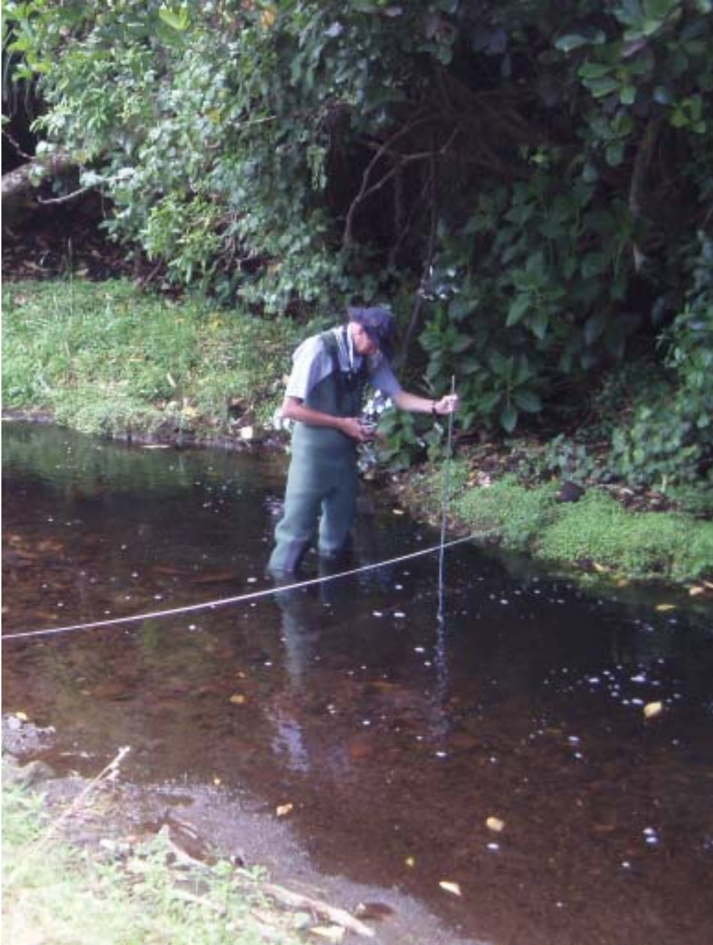
Photo 5 Streamflow measurement using a wading rod and propeller
