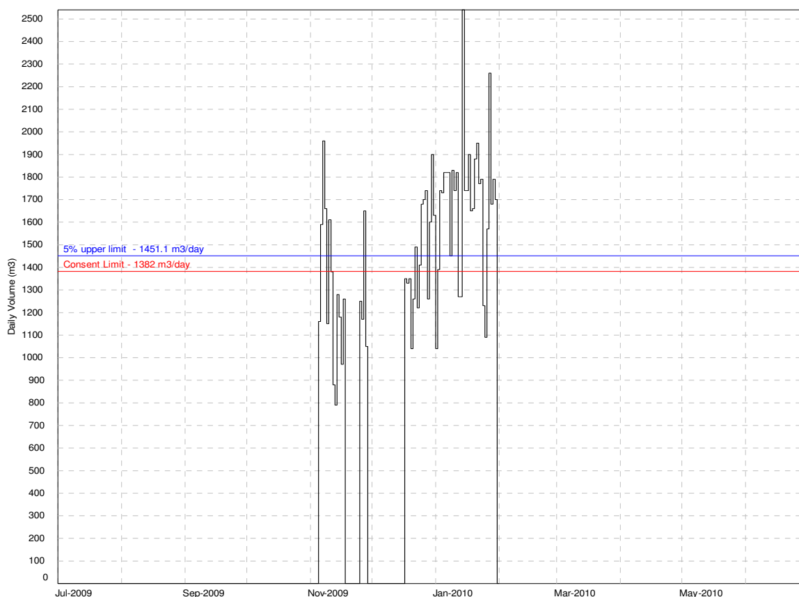
Figure 12 Amounts and dates of exceedance of daily volume of abstraction for consent 7243
