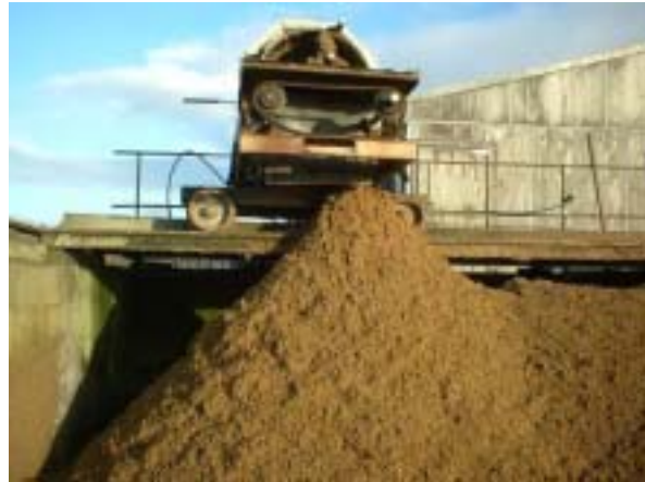
Photo 1 Solids separator and collection system
