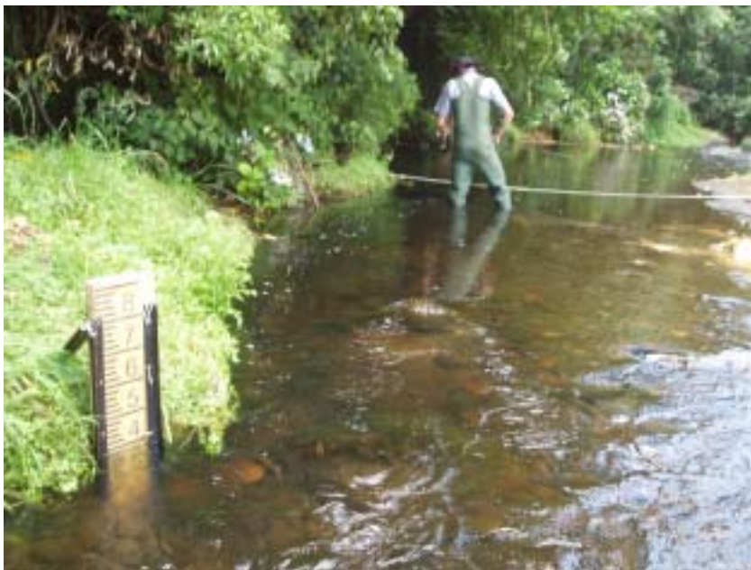
Photo 5 Streamflow measurement using a wading rod and propeller
