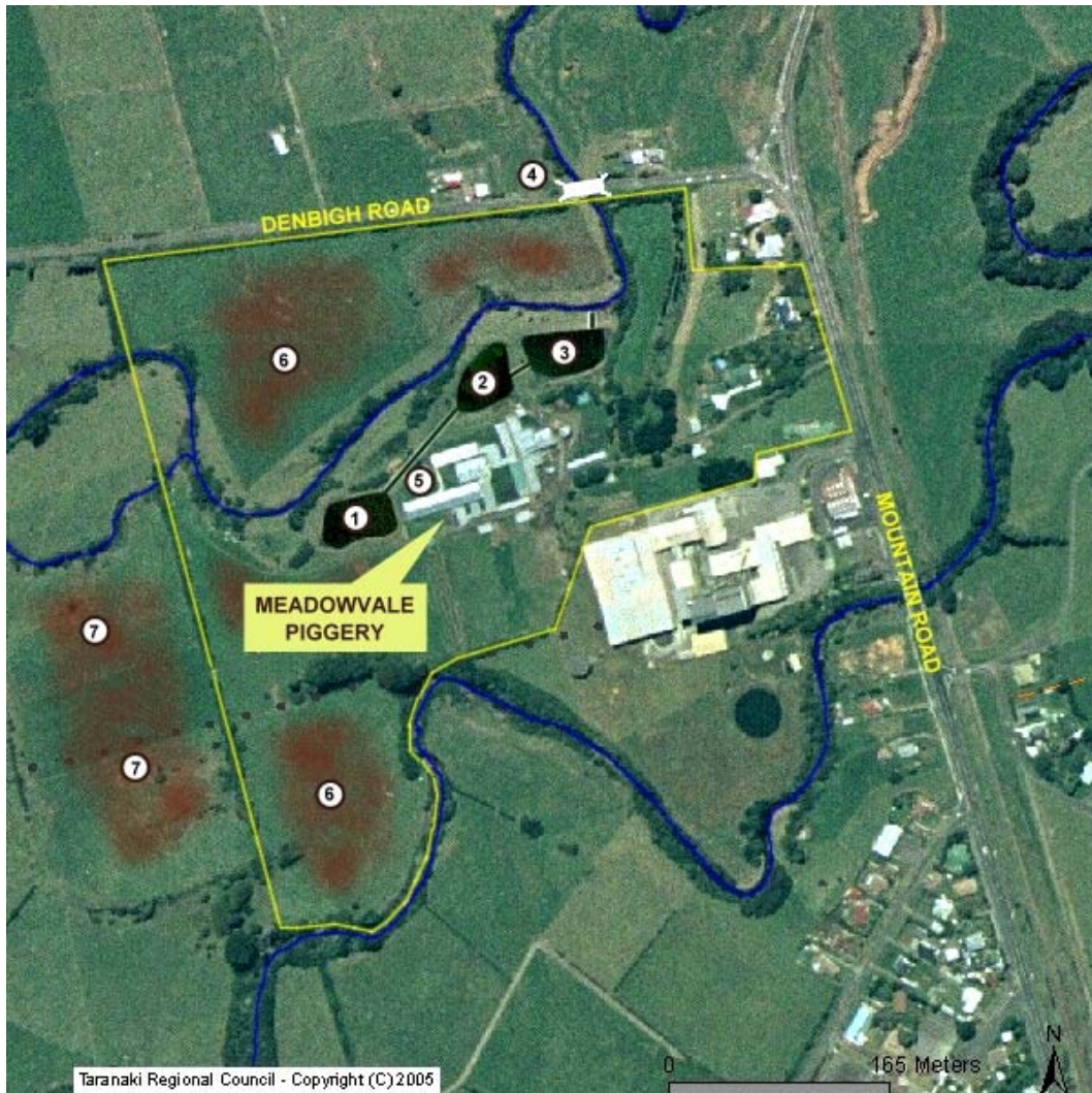
Figure 1 Piggery and disposal system
