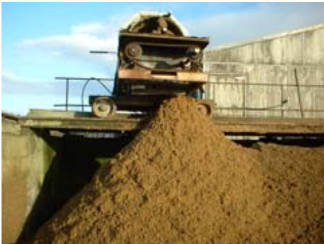
Photo 1 Solids separation and collection system.
