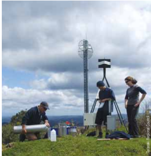
The Omahine rainfall recorder at Moana Trig helps provide flood warning for the Waitōtara Catchment.
