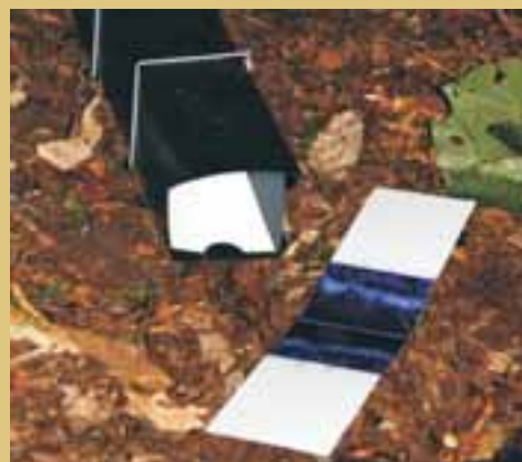
The ink card is placed in the tracking tunnel along with something tasty to lure the animal in. The tell-tale footprints left behind provide the clues as to the animal's identification.
