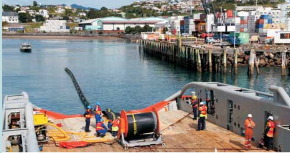
TRC and Port staff deploying the boom during a recent oil spill exercise.
