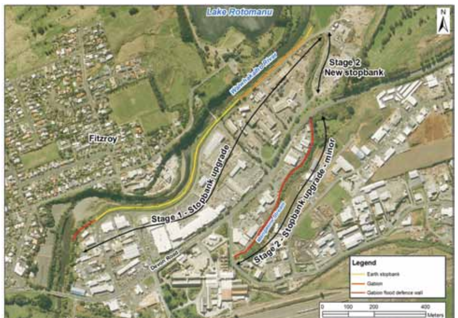
An overview of Stages 1 and 2 of the project.
