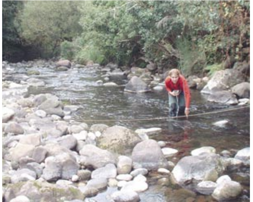
Fiona Moore, Hydrological Assistant, gauges the Patea River in Stratford. The flow is well below the mean annual low flow of 803 litres per second.
