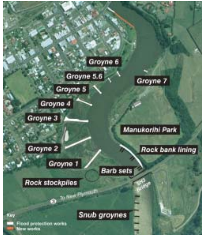
Figure 2: Waitara Flood Protection Scheme – adjacent to the SH3 Bridge
