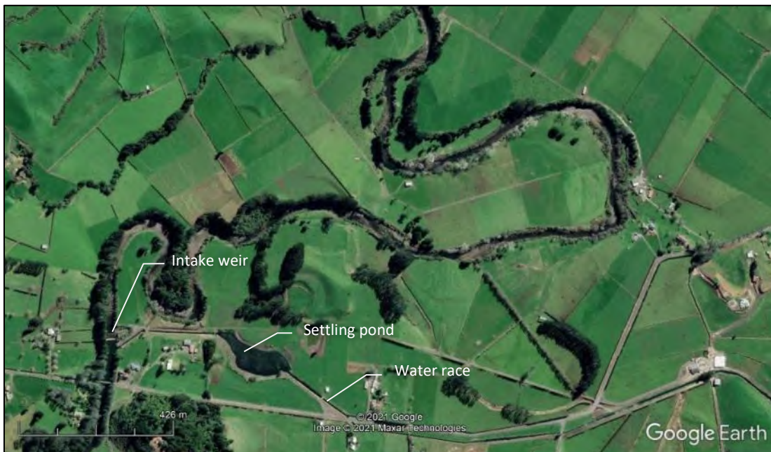
Figure 3.2 Aerial view of landcover in the vicinity of the Motukawa intake weir on the Manganui River, the Motukawa water race, and settling pond.
