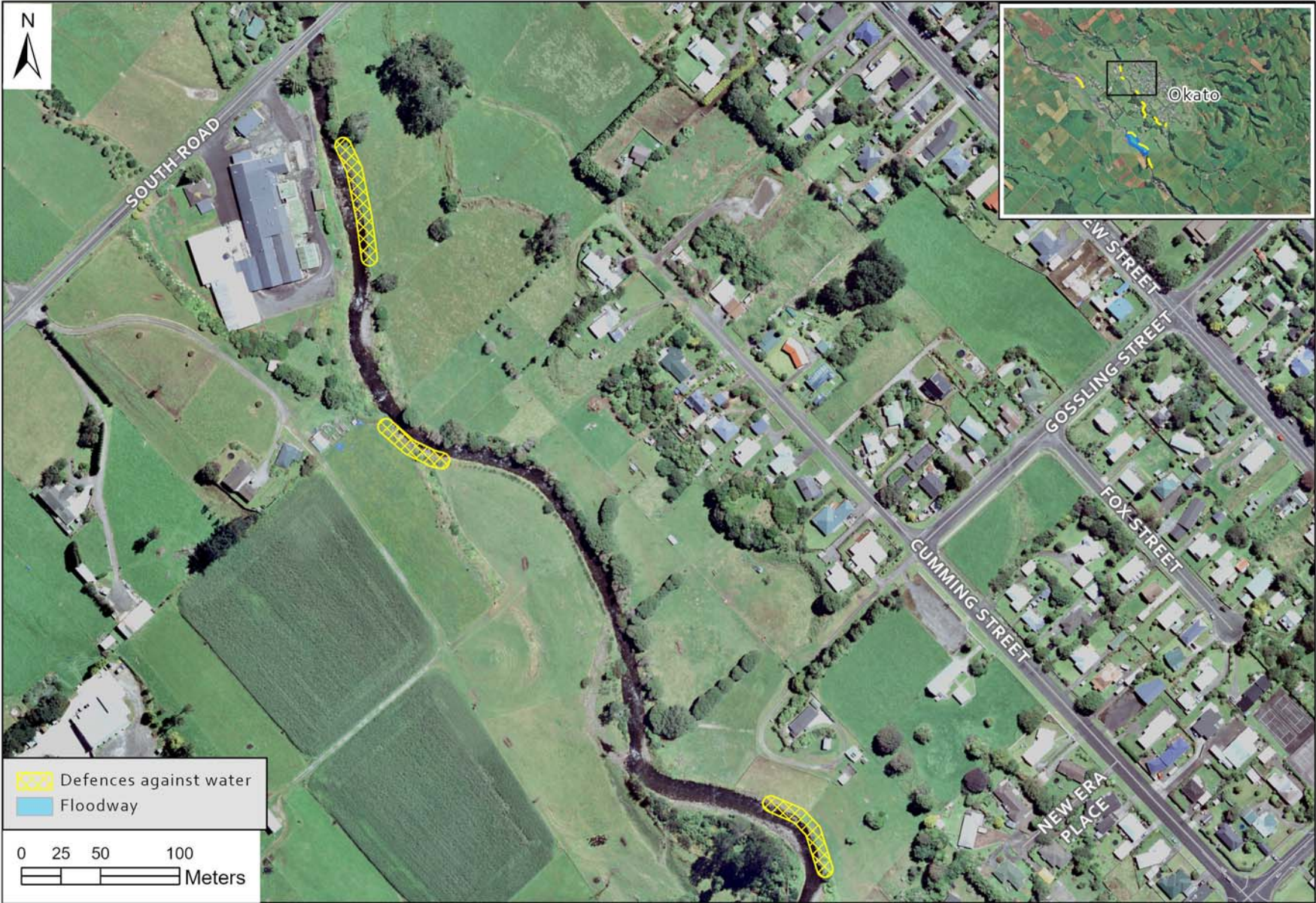
Map 4a Defences against water along the Kaihihi Stream, Okato. TARANAKI REGIONAL COUNCIL RIVER AND FLOOD PROTECTION BYLAW 2020
